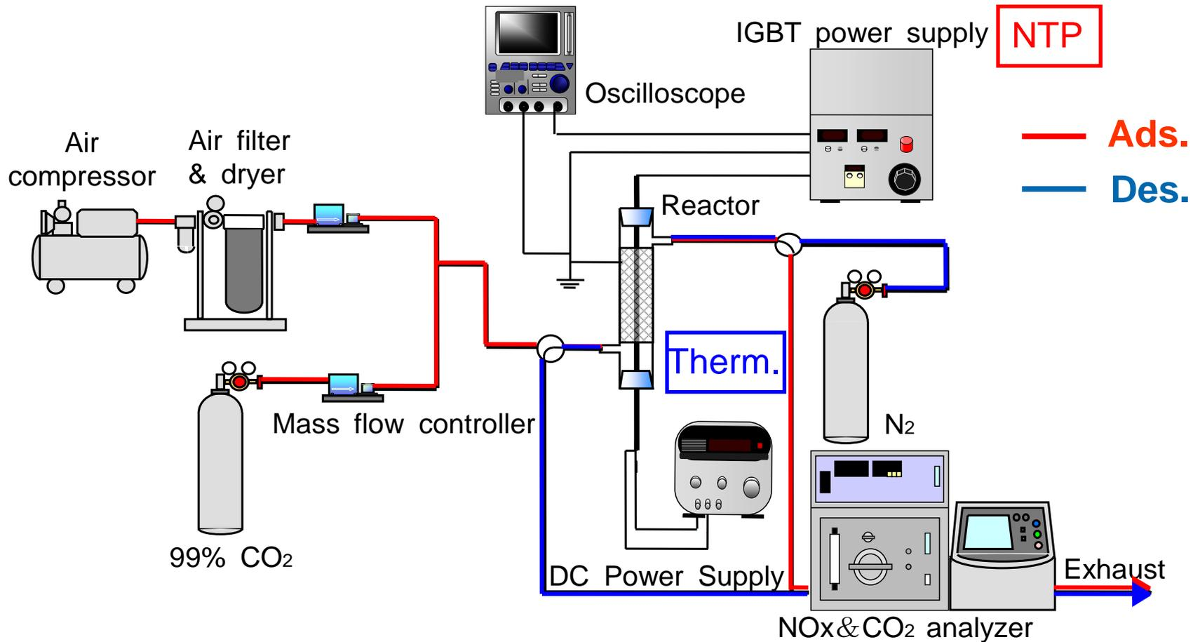
**Adsorption:** MS-13X (2mm, 12 g), CO<sub>2</sub> = 2.75%, Q = 4.0 L/min, t = 10 min
